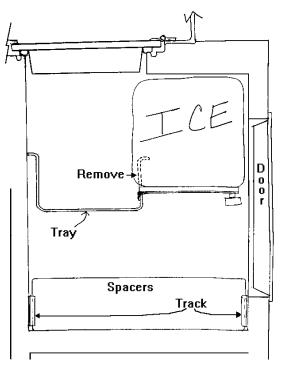
Additional insulation has been installed. An extra two inches of Styrofoam was added to the side and bottom areas of the ice box in the engine compartment and to the side in the forward part of the port seat lockers.
